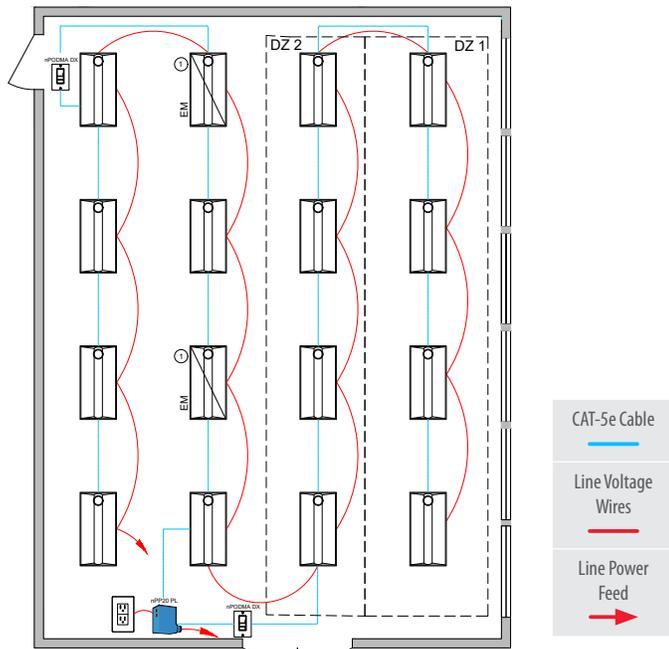
Ⓞ Some nLight enabled EM fixtures require a normal sense line connection. Wiring shown assumes battery backup emergency option. See fixture spec sheets for details.
