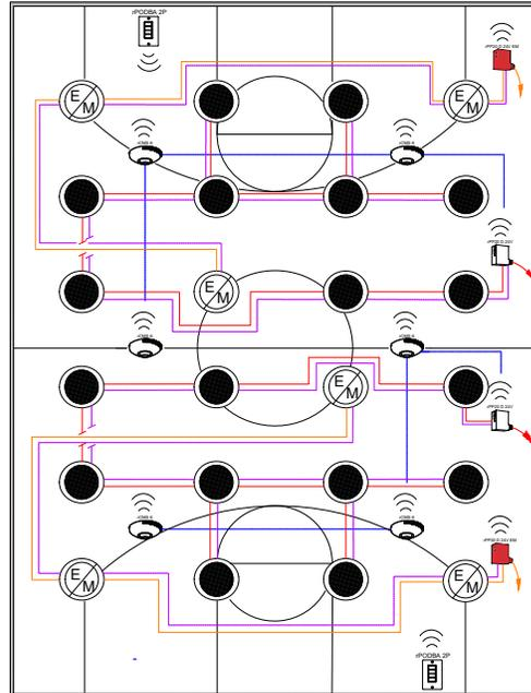
① Fixture(s) assumed to include power interruption detection emergency option. For battery backup option, no dedicated EM circuit necessary.
