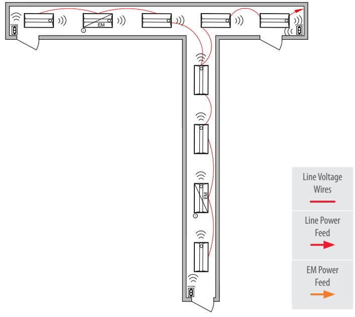
① Some nLight enabled EM fixtures require a normal sense line connection. Wiring shown assumes battery backup emergency option. See fixture spec sheets for details.
