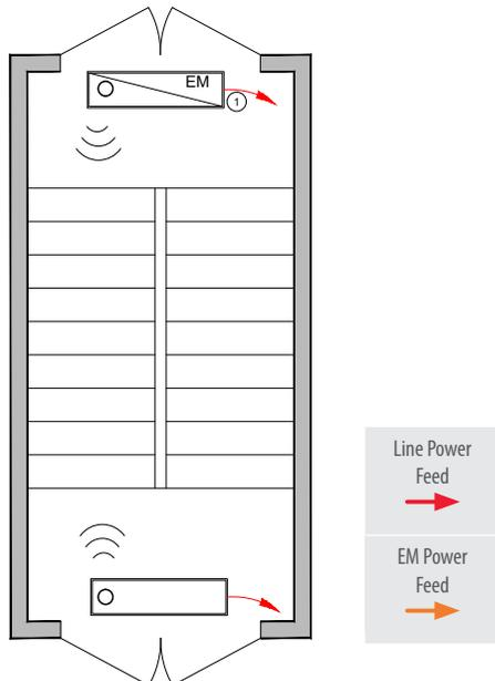
① Some nLight enabled EM fixtures require a normal sense line connection. Wiring shown assumes battery backup emergency option. See fixture spec sheets for details.
