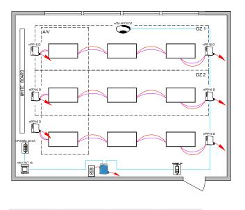
CAT-5e Cable Line Voltage Wires Line Power Feed 0-10V Wires
