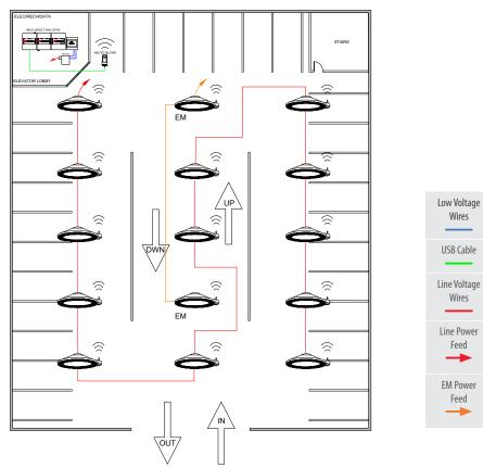
⑦ Fixture(s) assumed to include power interruption detection emergency option For battery backup option, no dedicated EM circuit necessary.
