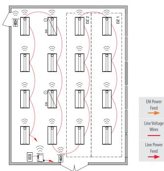
① Some nLight enabled EM fixtures require a normal sense line connection. Wiring shown assumes battery backup emergency option. See fixture spec sheets for details
