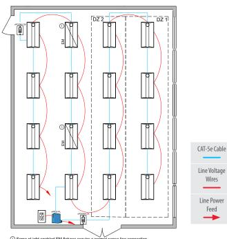
O Some nLight enabled EM fixtures require a normal sense line connection. Wiring shown assumes battery backup emergency option. See fixture spec sheets for details
