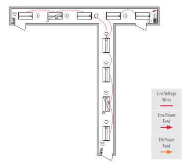
O Some nLight enabled EM fixtures require a normal sense line connection. Wiring shown assumes battery backup emergency option. See fixture spec sheets for details.
