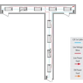
O Some nLight enabled EM fixtures require a normal sense line connection. Wiring shown assumes battery backup emergency option. See fixture spec sheets for details.
